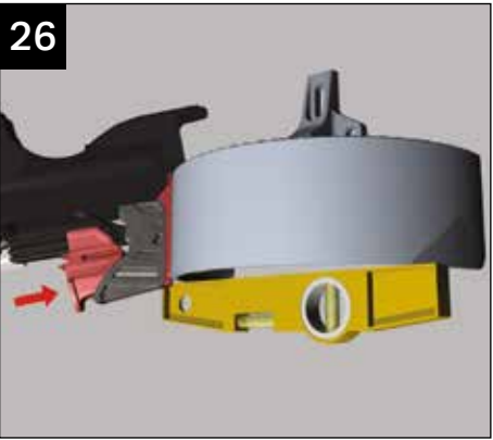
Finally when all is level and plumb, use your thumb to push up all the lower wedge locks. The roof is now set. Now return to fasten the frames to the host wall and the dwarf wall.
