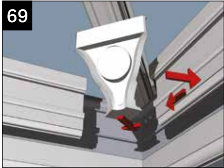
Slot each section of internal fascia into the corner jointer and tap the fascia onto the barbs of the eaves beam. Fit Ultraselect strips into the slots in the fascia
