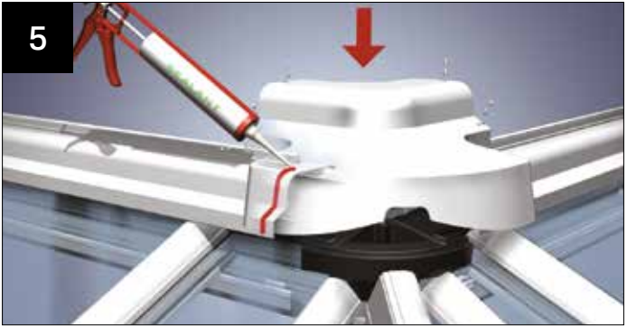
Now, as per main guide, seal around each glazing bar top cap where it meets the inner wall of the 'soft touch' weathering shield. Take the length of PVCu ridge top cap assemblies, seal the two ends to be joined. Mark and drill for final rivet positions using a 5mm drill bit. Apply plastic rivets. Offer the whole assembly into position, trimming may be required - see over page. The trimming should be in the form of removing a strip across the whole width or as shown above, notching around each bar. Secure ridge into position with 'T' bolts as shown in section 4.
