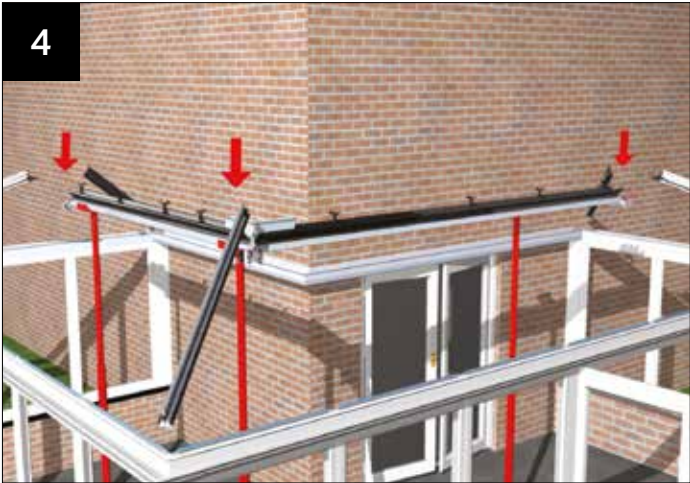
Temporary support/prop the 'L' shaped ridge. Offer up the hip bars. Secure using steps 12-15 in the main installation guide. Build remainder of the roof as section 4.
