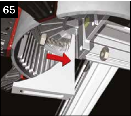
Fit the "L" shape PVC bracket to the underside of the radius end. Offer up the internal radius end to check the position of the bracket before tightening.
