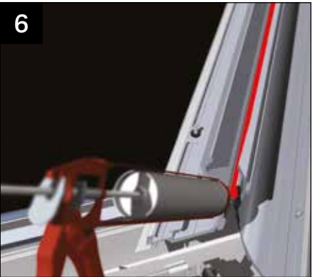
Now run a continuous bead of suitable silicone down the entire length of the aluminium valley profile, at the point of the hinged connector in the centre.
